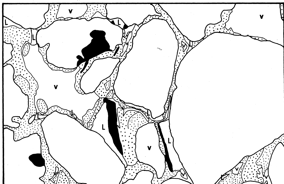
FIGURE 11. Photomicrograph (top) and interpretative diagram (bottom) of limpid clay coatings around sand grains which are postdated by complex speckled-impure clay coatings in thin section 1 e. PPL; HFL = 1.3 mm (key as for figure 4b).
